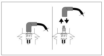
Figure 3. Disconnecting/Connecting Spark Plug
